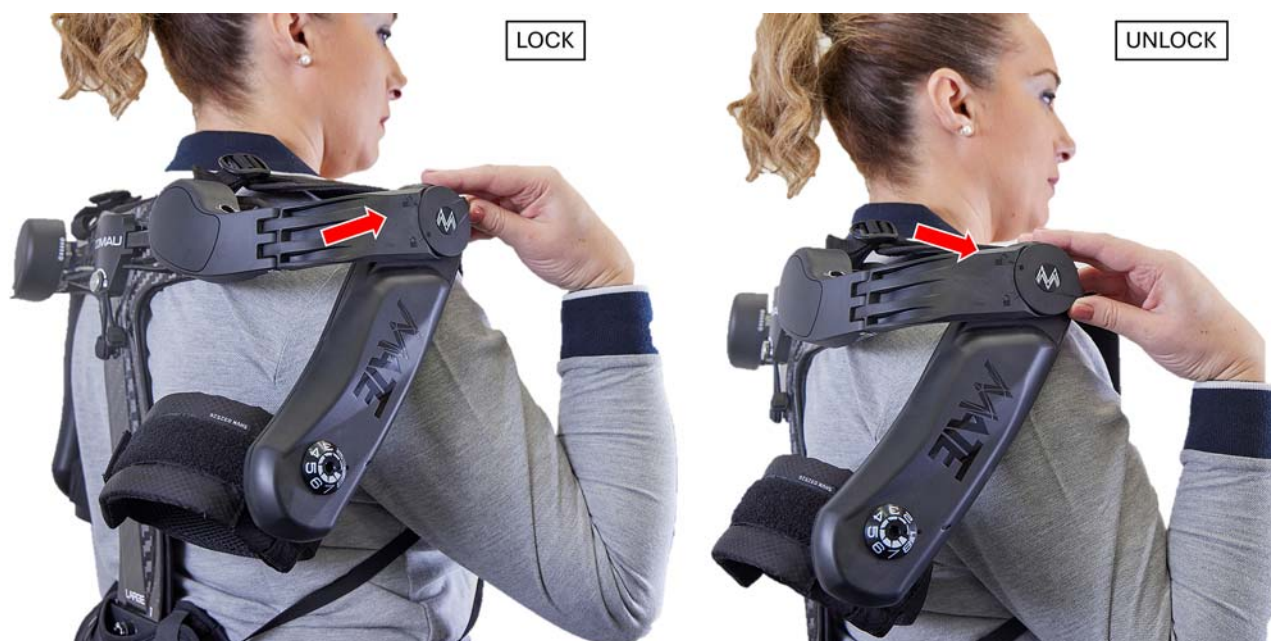
Fig. 3.6 - Torque Generating Box (TGB): locking mechanism
