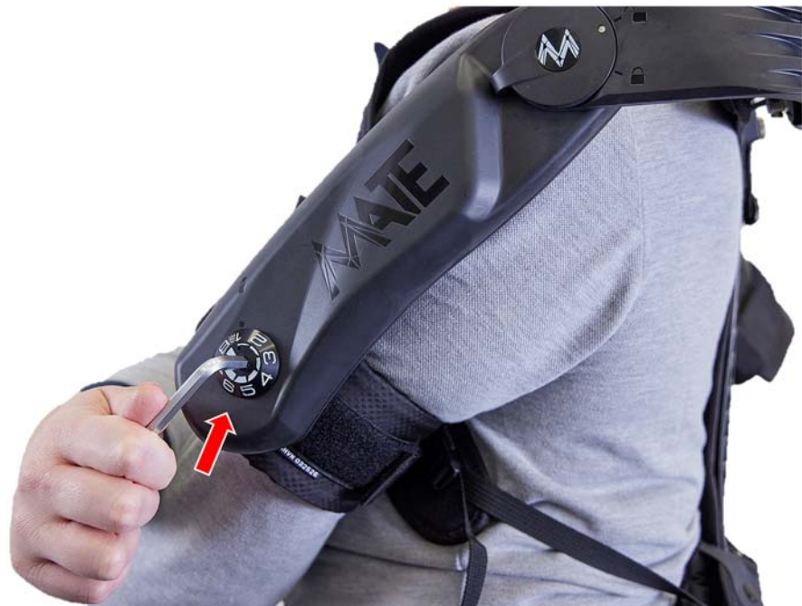
Fig. 4.3 - Close-up view of the adjustment site on the Torque Generating Box and assistance level indicator
