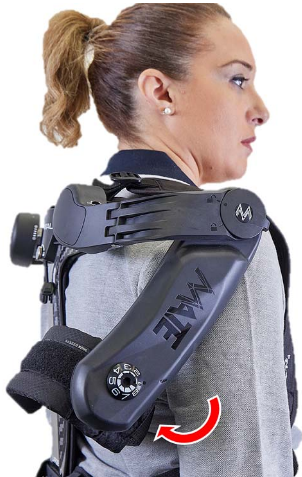
Fig. 3.5 - Torque Generator Box in rear rest position. This is the only position where the locking mechanism can be activated or deactivated
