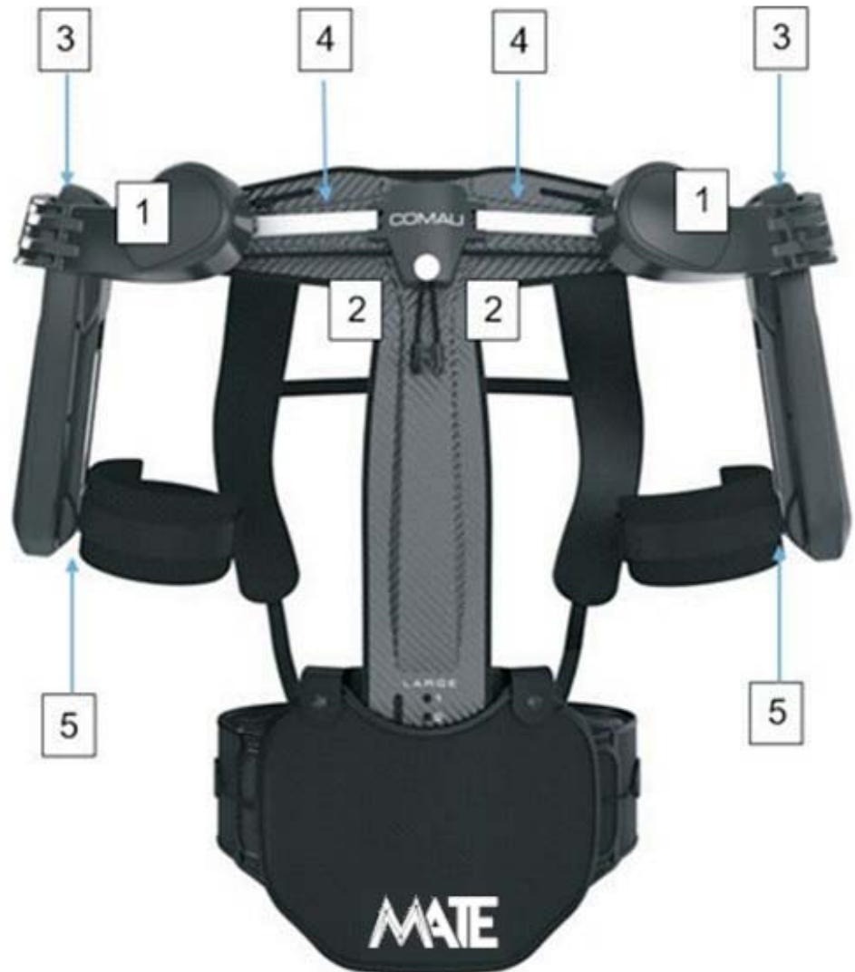
Fig. 3.3 - Passive degrees of freedom (pDOFs)
