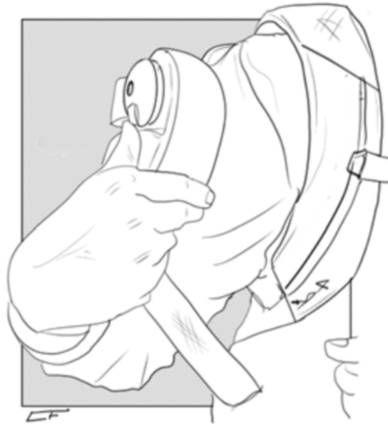
Fig. 5.14 - Locking the Torque Generating Box lock mechanism.
