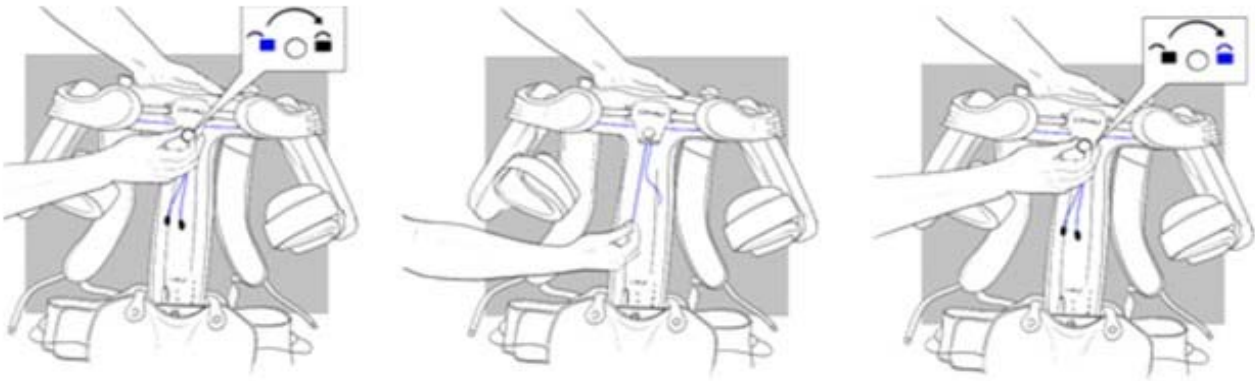
Fig. 4.2 - How to adjust the rear elastic bands
