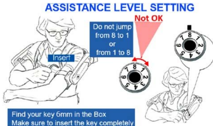
Fig. 4.4 - Assistance Level Setting
